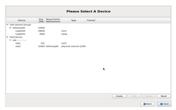
Above screenshot displays default partitioning schema, which needs to be changed to be suitable for Enigma NMS.
