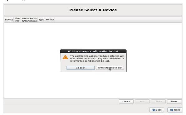
Click on **Write changes to disk** button, after which you will see how system creates and formats new file system partitions:
